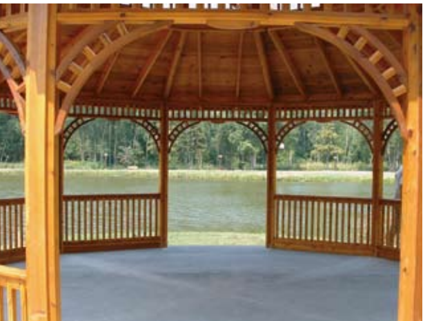
Our 23', 12-sided Pavilion includes an all clear span ceiling, 2x6 western red cedar rafters with 1x12 knotty cedar ceiling, cedar shakes and cedartone exterior stain.
